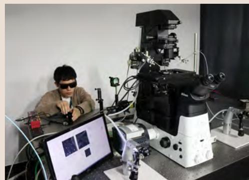
光検出磁気共鳴(Optically Detected Magnetic Resonance)顕微鏡
